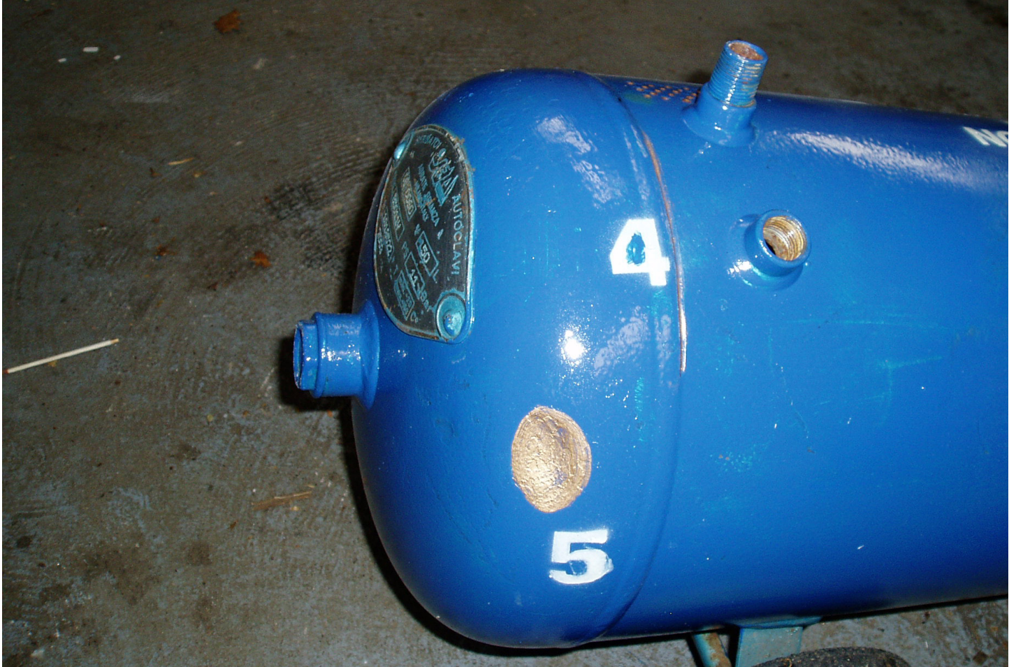
PHOTO 4,5: WELD GRINDING MARK (4) AND HEAD DENT (5)
