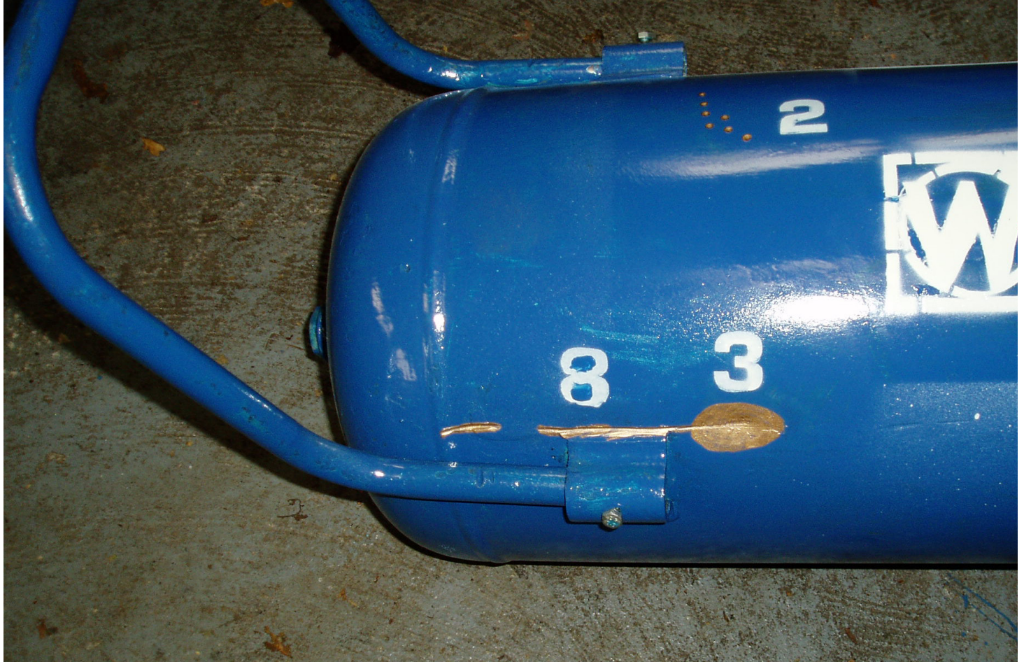
Dent size 45mm x 20mm x 2.5mm deep. Smooth edges
