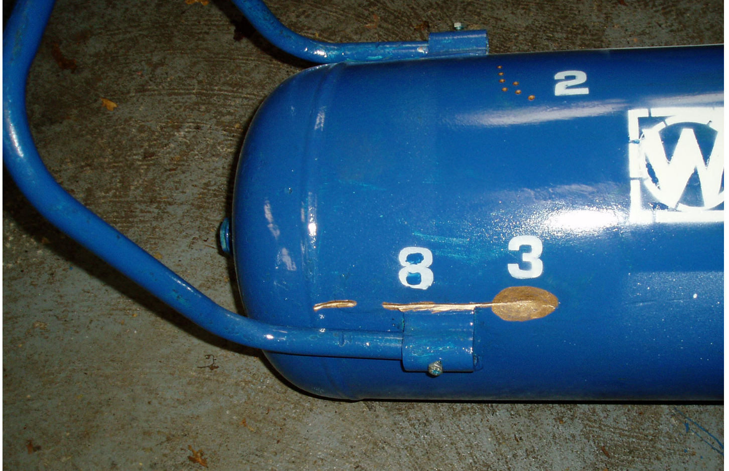
PHOTO 8: SHELL GRINDING MARKS
