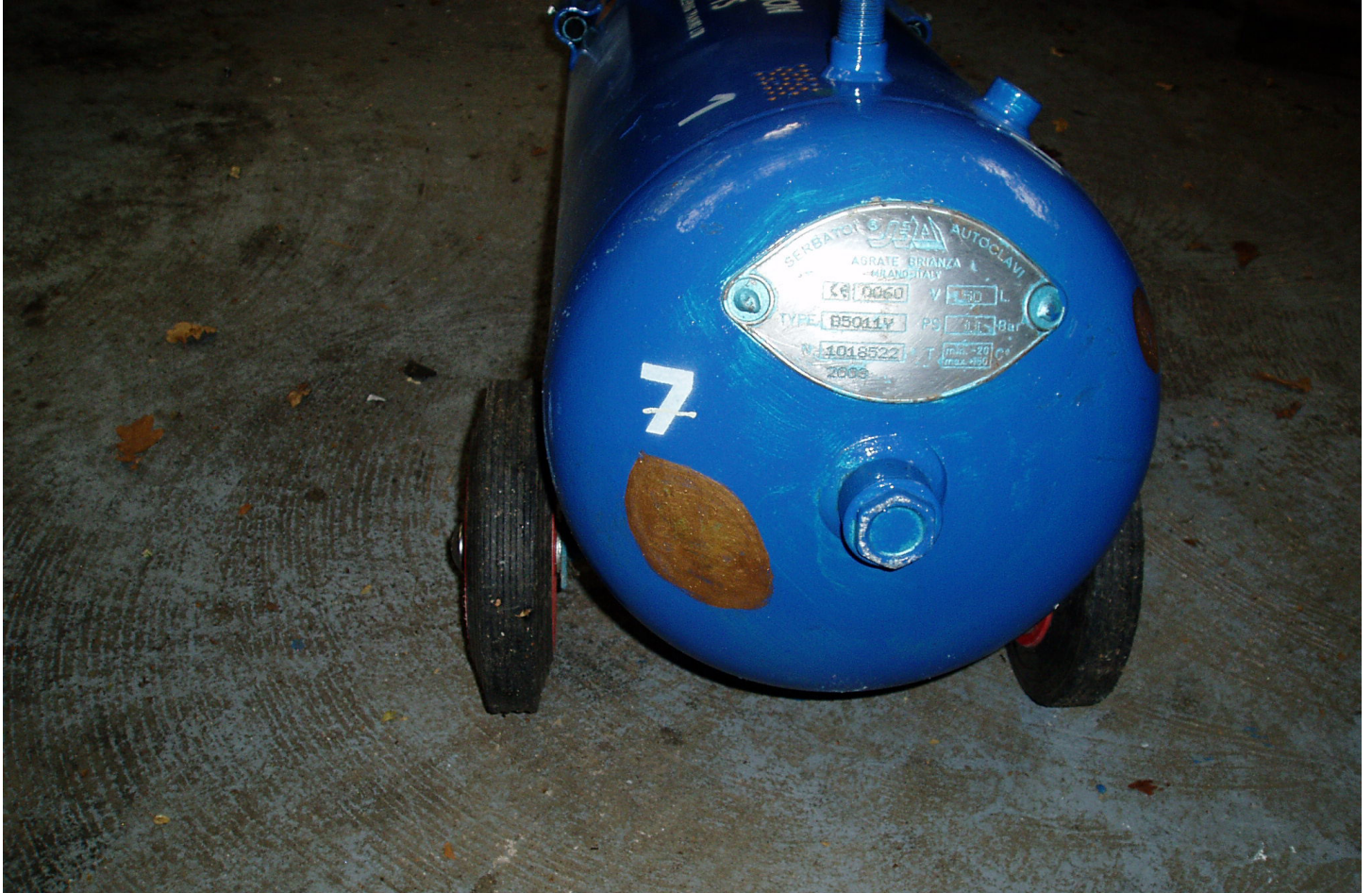
PHOTO 7: HEAD WALL THINNING (NAMEPLATE END)
