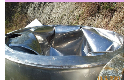
The replacement vessel after buckling failure of the internal annulus
